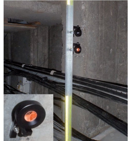
Left: Carrying out the blind wire test. Right: Total station prisms inside the box monitor movement.
